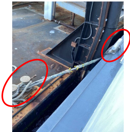
The line was pre-made to a bit on the pier and of a fixed length. Crew removed the eye and hung it on a pier-side hook for ease of access.
