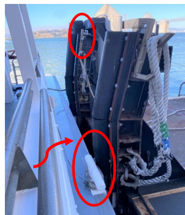
Crew stood sideways on this outboard gunwale to handle the aft spring line. The cleat was hard to access and outboard of the railing. The hook used is also pictured.
